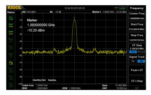
Note that the marker above shows the peak at 1GHz with an amplitude of -10dBm.
