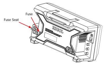
Figure 1-16 To Replace the Fuse
