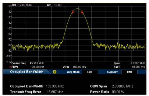
Figure 2-17 OBW Measurement Interface
