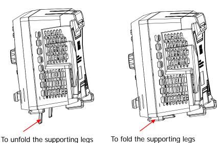
Figure 1-3 To Adjust the Supporting Legs
