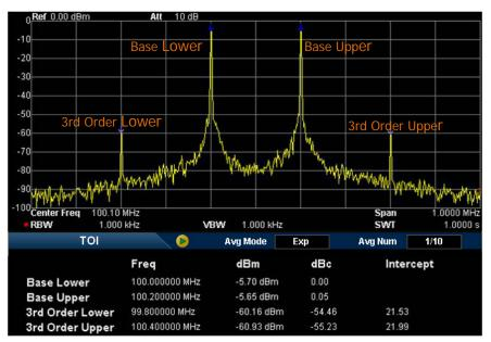
Figure 2-21 TOI Measurement Interface
