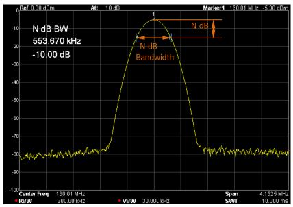
Figure 2-25 N dB BW measurement
