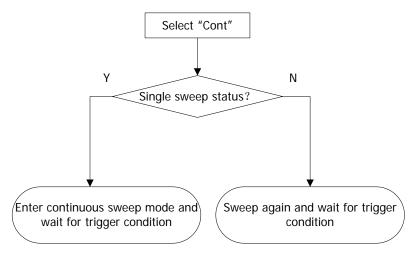
Figure 2-9 Process of Continuous Sweep
