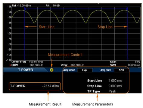
Figure 2-14 T-Power Measurement Interface
