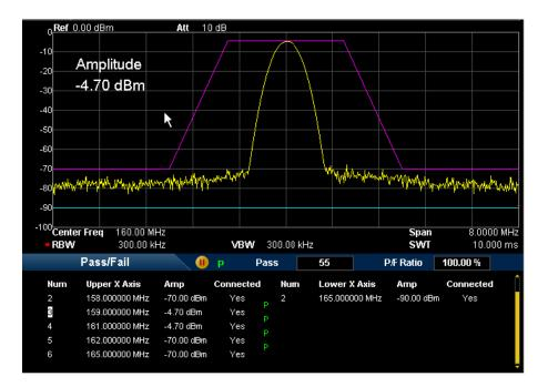
Figure 2-11 Interface of Pass/Fail Test
