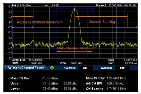
Figure 2-15 Adjacent Channel Power Measurement Interface
