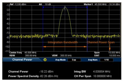
Figure 2-16 Channel Power Measurement Interface
