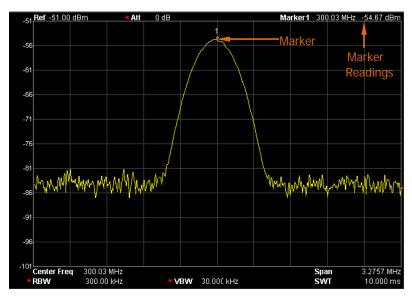
Figure 2-23 Schematic of the Marker
