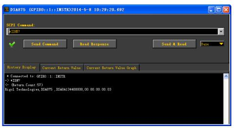
Figure 3-9 Write and Read Commands via GPIB
