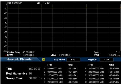
Figure 2-20 Harmonic Distortion Measurement Interface
