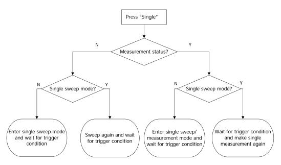
Figure 2-10 Process of Single Sweep
