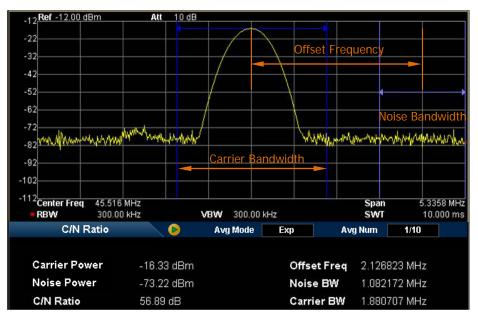
Figure 2-19 C/N Ratio Measurement Interface
