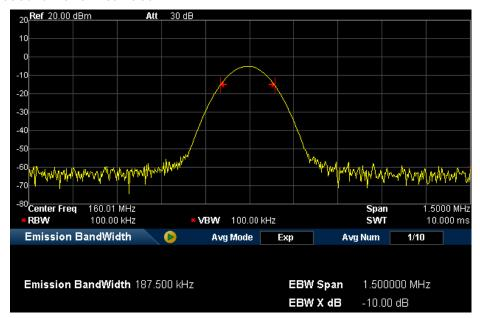
Figure 2-18 EBW Measurement Interface
