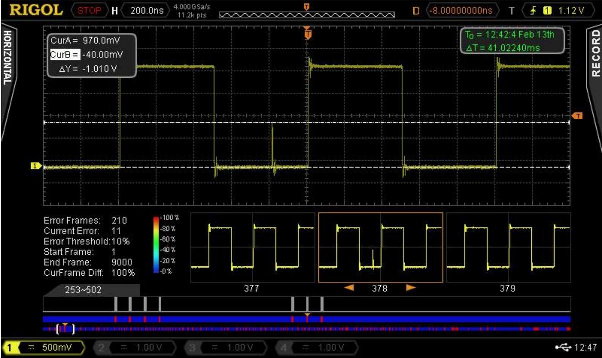
The third and most advanced alternative is the combined usage of the record function and the available trigger functions. The oscilloscope can be configured in that way, that only the error is recorded. Depending on the frequency of error occurrence and time base settings it is possible to monitor the signal and record the errors up to hours.
