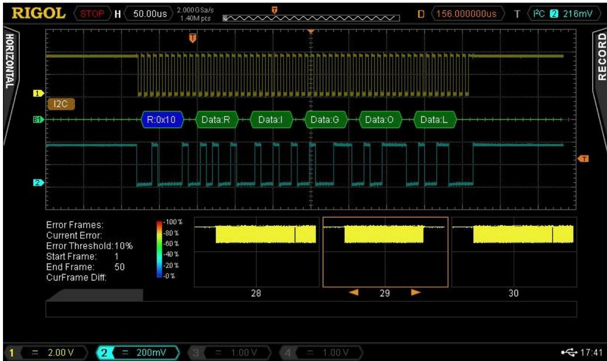
This function is not only usable to separate the data traffic on serial busses with addressing, it can also be used to locate errors in data transmissions. Depending on the bus it is also possible to trigger directly on error frames and record the corresponding frame and analyze it afterwards and solve the issue.
