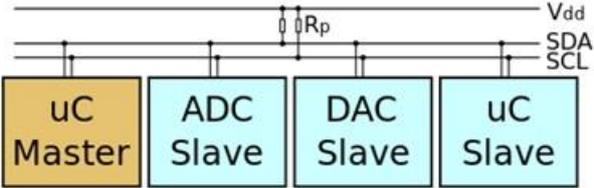
The member selection at I<sup>2</sup>C Bus is realized with the existence of an address section which is transmitted in the data package, not as hardware selection line like at the SPI Bus (called Chip Select or Slave Select). To filter out and monitor only the messages of one specific
