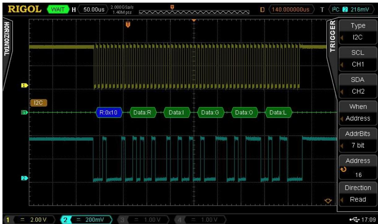
The screenshot above shows a single decoded message. The data traffic on the bus could be high so that the time between the messages between master and slave with address 16 could be very long. How can it now be achieved that the messages between Master and „Slave 16“ are separated and being displayed in a compact manner, without the need of sorting out many of not wanted messages by hand?
