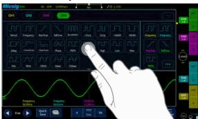
Swipe downward from the top edge of the screen to immediately access 31 types of measurement options in one time.
