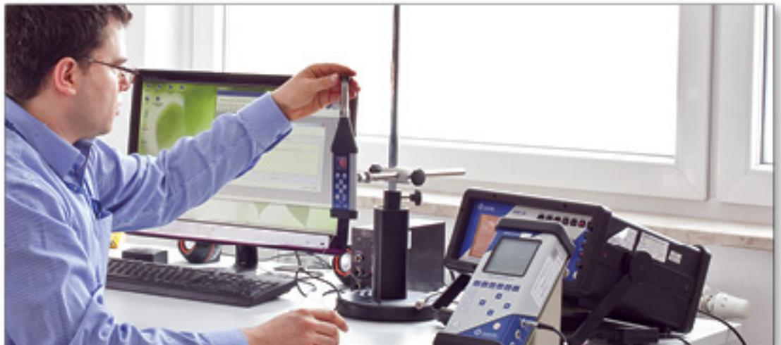
The SVAN 971 is a full class 1 instrument that has options for octave and third octave band filters. It has a measurement range of 15dB to 140dB which gives an incredible dynamic range that's greater than 110dB. It can record audio comments to .wav files and measures both SLM (sound level meter) and dosimeter data. The instrument has many unique features, like peak spectrum, that put it out there in a class of its own.
