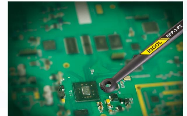
NFP-3-P4, a near-field probe which resolution is 2 mm. It can detect the vertically emitted electromagnetic field. It is applicable for the detection of magnetic field where current loop exists. For example, electromagnetic field testing for PCB wiring, magnetic field testing for IC pins area etc
