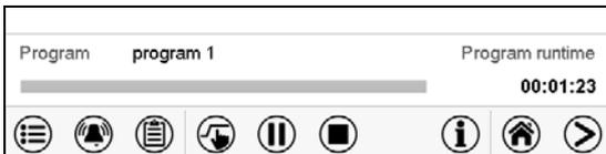
Normal display. Information on the bottom of the screen indicates the currently running program and the time already passed. The grey bar shows how much time of the whole time is elapsed. If program duration has been set to infinite, the grey bar is not displayed.
